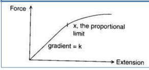
On graphs showing force against extension, you can see when the limit of proportionality is reached by looking at where the graph starts to curve. (Labelled x on this example)
