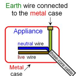
The live wire is the most dangerous one, since it is at 230 V. it should never touch the earth wire (unless the insulation is between them, of course!), because this would make a complete circuit from your mains supply to the ground (earth). A shock or fire would be highly likely.
