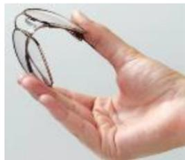
**Shape Memory Alloys** change shape easily but always return to their original shape when they are heated. There are many applications such as dental braces and unbreakable spectacles.
