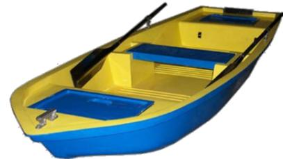
**Glass reinforced plastic (fibreglass)** is made from fine glass fibres which are combined with a thermoset plastic resin and is moulded. It has a very high strength-to-weight ratio, resists corrosion, water resistant and is light weight. The fibre glass fibres are soaked in liquid plastic, and then pressed or heated until the material fuses together.
