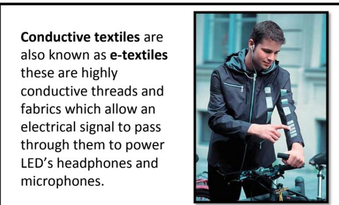
**Conductive textiles** are also known as **e-textiles** these are highly conductive threads and fabrics which allow an electrical signal to pass through them to power LED's headphones and microphones.
